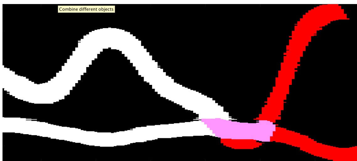
Figure C.5: Using the Retrieve Original Image tool (second from left), the overlapping region has been defined here and as a result has turned pink, and the surrounding objects reclassified.
